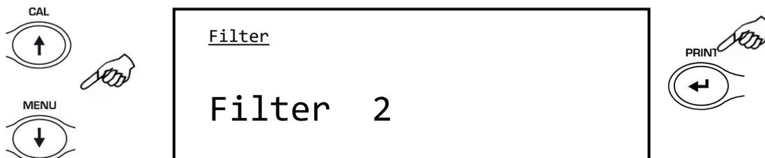
2. Select the desired filter level. Pressing the **MENU** or **CAL** button it will be possible to scroll through the various levels forward or backward; then confirm your choice with the **PRINT** button.
